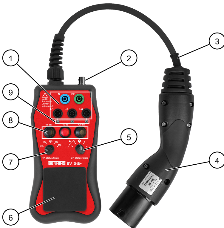
Figure 1: BENNING EV 3-2+ device structure
