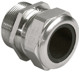
AGRO Kabelversch. PROGRESS MS M25 Kabel Ø 12.5-20.5mm (UL 14.5-16.0)
