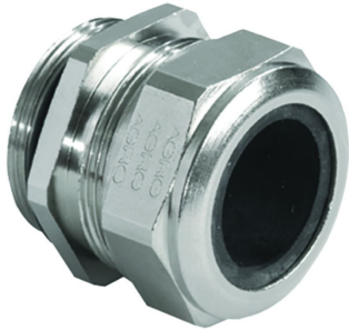
AGRO Kabelversch. PROGRESS MS Pg9 Kabel Ø 3.5-4.5 mm (UL 4.5-4.5)
